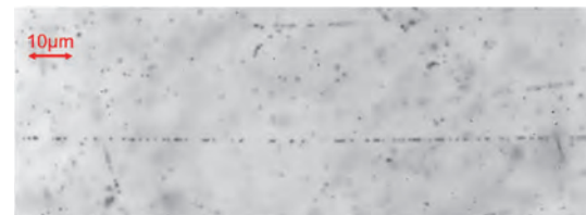
Fig. 2. Optical microscopic image of electron beam (several tens of MeV) track. The electron beam was exposed at UVSOR.
